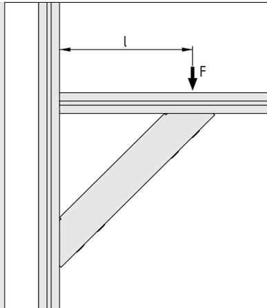
$$F < 1000 \text{ N} \wedge F \times l < 300 \text{ Nm}$$
