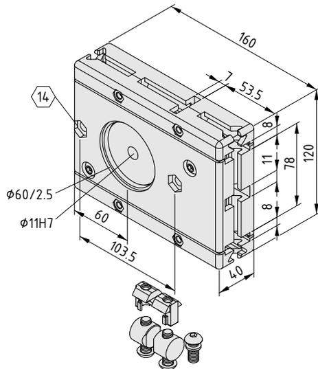
**Zahnriemenumlenkung 8 80 R25 mit Bohrung**
